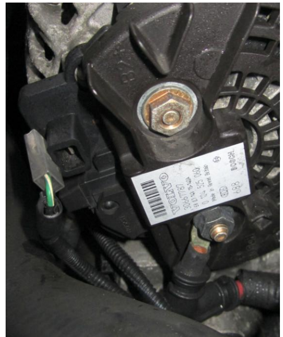
Control Cable Removed
