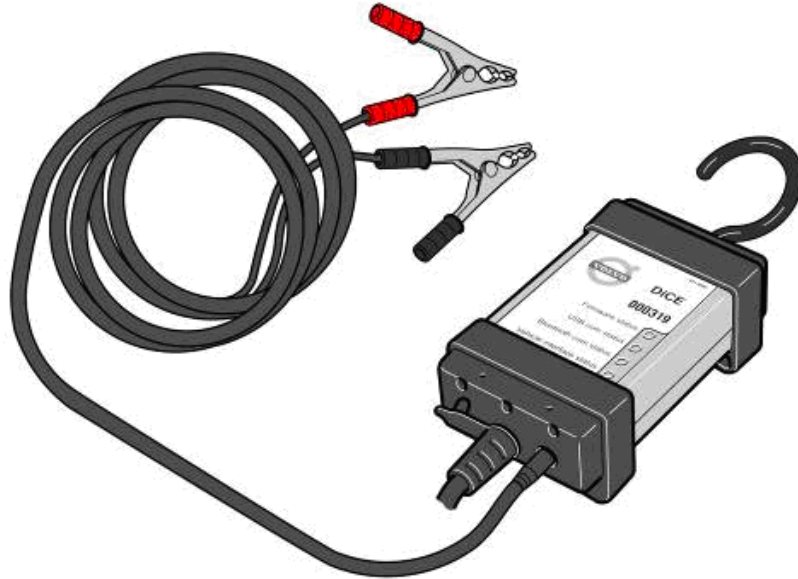
Fig. 16 Battery cable attached
