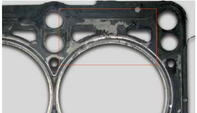
▲ Elastomer coating damaged by overheating
