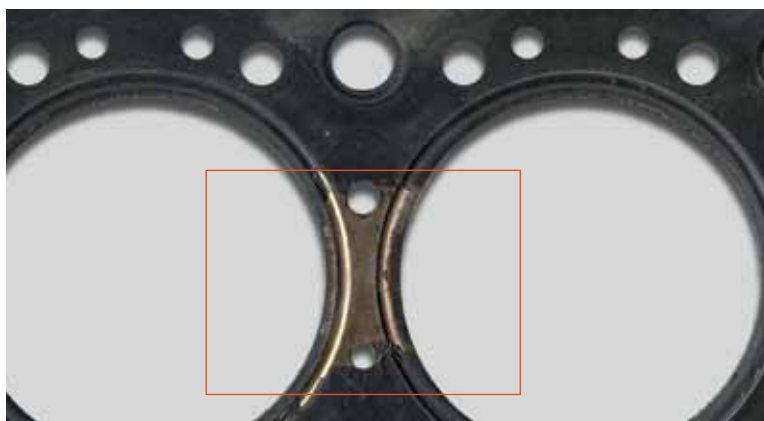
▲ Scorched elastomer coating
