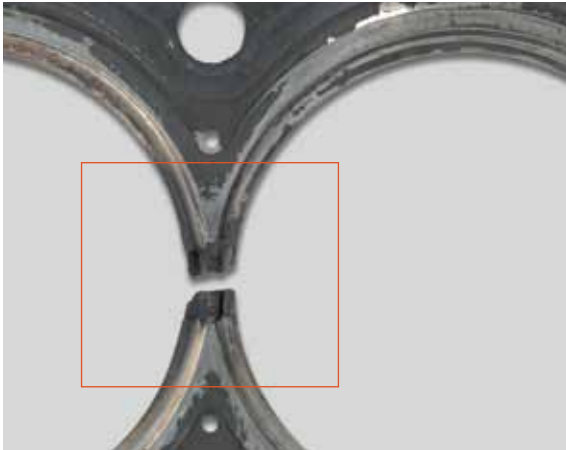
▲ Broken web caused by high component dynamics
