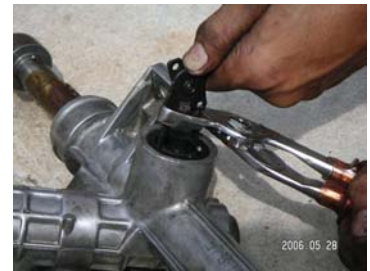
PIC 10: Removing the rear plug
