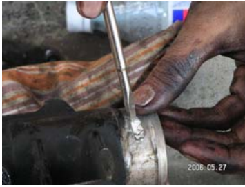
PIC 8: Opening filled with silicone
