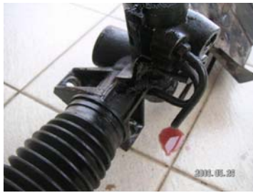
PIC 3: Main leaking points
