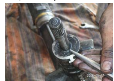
PIC 7b: Marking the starting point on the pinion
