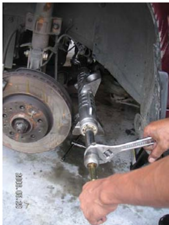
PIC 5: Removing the inner rod
