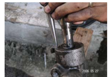
PIC 7a: Marking the starting point on the pinion housing
