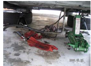
PIC 1: Support the car with 2 jack stand, with hydraulic jack supporting the transmission body
