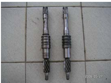
PIC 12: Serviced pinion vs. the stock
