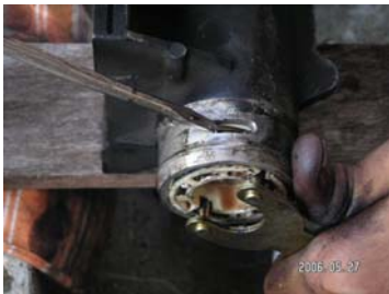
PIC 9: Removing the locking pin
