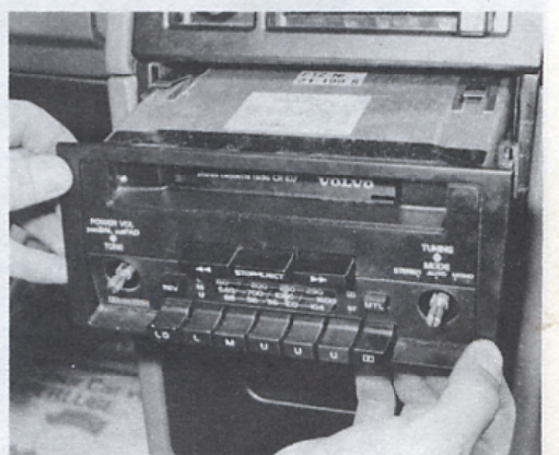
35.4C Removing the radio/cassette unit
