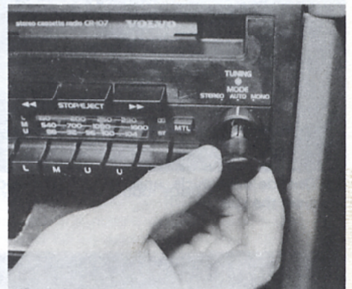
35.3 Pulling off a radio knob
