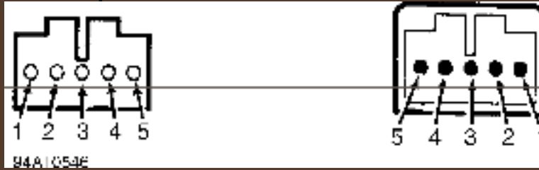
Fig. 6: Identifying Passenger Compartment Temperature Sensor Connector & Component Terminals Courtesy of Volvo Cars of North America.
