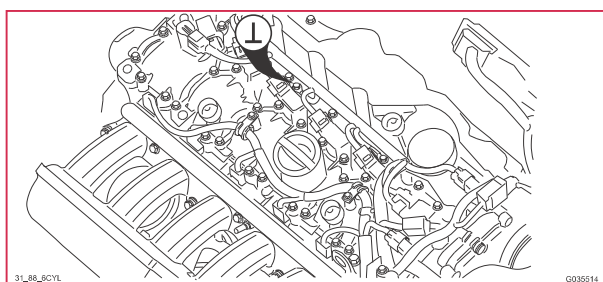
31/89 Ground connection, Engine ignition coils, 5-Cyl.
