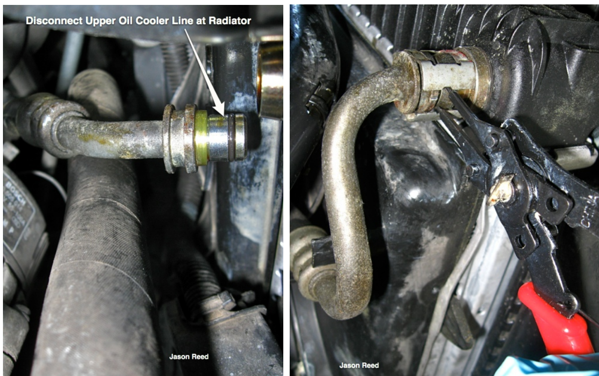
Left: Upper line disconnected. Right: Lower line clamp being spread with pliers.
