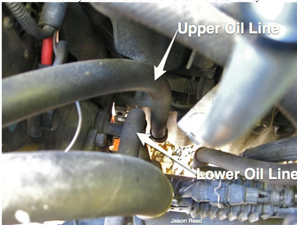
General routing pathway for the upper and lower oil lines.
